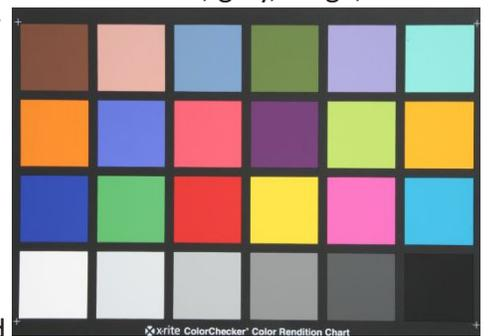
Fig. 2. X-rite color calibration chart used to correct the color variations in the images
