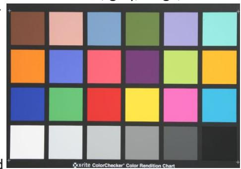
Fig. 2. X-rite color calibration chart used to correct the color variations in the images
