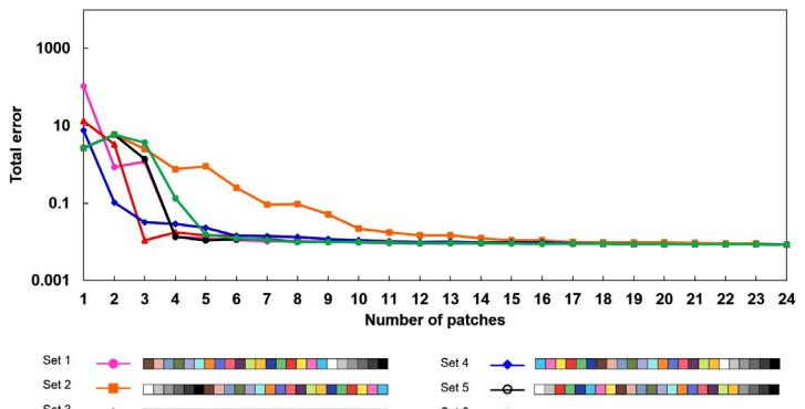
Fig. 4. Relationship between number of color patches and error produced during color calibration
